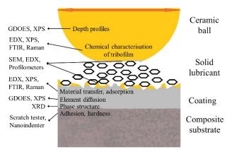
The proposed work will apply thin protective coatings, deposited by means of vacuum methods (PVD), as anti-wear and anti-oxidise coatings, and a solid lubricant, applied as component of composite or external, at surface, to reduce the coefficient of friction.
