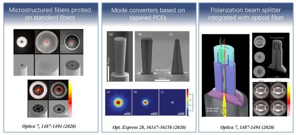
The new types of fiber optic devices proposed in the project (as mode converters that can be adjusted, broadband fiber-integrated mode splitters that can split light into different modes, and switchable fiber-integrated vortex beam generators) could be used not only in telecommunication systems but also in super-resolution microscopic imaging, optical trapping and fiber-optic sensing.
