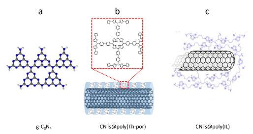
Schematic showing the structure of (a) a carbon nitride,  $g-C_3N_4$ , (b) a carbon nanotube with a thin polymeric film of catalytic porphyrin centers deposited inside the polymer, and (c) a carbon nanotube with a thin film of ionic liquid-based polymer deposited on its surface.
