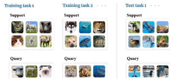
Figure 1: We present a visualization of a few-shot learning problems. During the training process, we update model parameters based on training tasks. After training, our model has to correctly classify the query set (from the test task) using the element from the support set.
