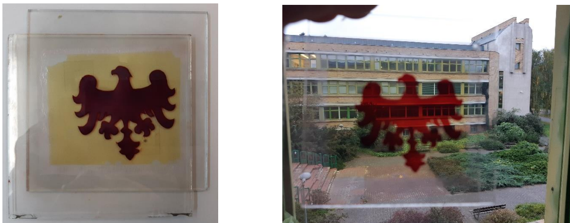
Fig. 1. Demonstration DSSC device with a single MK2 dye with dimensions of 10 x 10 cm made in our research group. On the left: active dye covers the surface of the eagle from the AMU logo, the rest is filled with electrolyte. On the right: a photo cell in front of the building of the Faculty of Physics, AMU.
