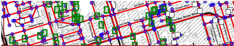
Figure 1: A sample agent based simulation state of a transportation system. Cars are marked with squares and intersections with circles.
