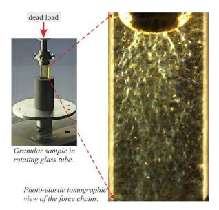
regardless of the external macro-scale conditions and they can be observed, described and modelled using the idea of photo-elastic optical tomography supplemented by discrete element method (DEM).
