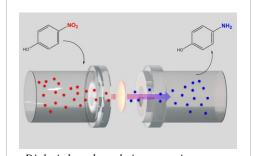
Dialysis based catalytic-separation system. System operates due to the pNCs membrane placed in the middle between two chambers. NARs in the left chamber are being reduced and transferred to the right chamber in form of AAMs
