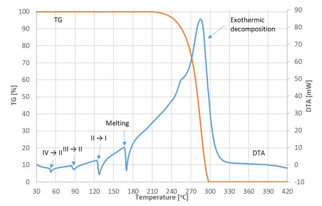
DTA-TG measurement results of ammonium nitrate sample, mass loss and phase transitions together with exothermic decomposition can be seen on TG and DTA curves, respectively.
