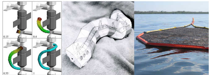
Fig.1. On the left: selected steps of continuous deployment of 40 Arm-Z modules to bypass Yarya module (shown in dark gray) of the International Space Station . Hue indicates the unfold angle for the individual units. Red and cyan indicate fully stowed and deployed positions, respectively. For each state the unfolding rate is shown in the bottom left corner. In the middle: conceptual visualization of Arm-Z habitat in extreme environment in “banana-split” orientation. On the right: An example of an oilspill boom system available at Canadyne Technologies .
