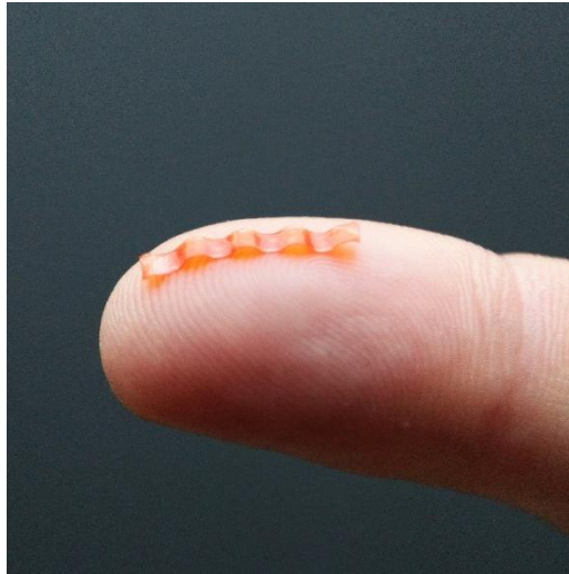
Fig. 1 A natural scale caterpillar micro-robot made of liquid crystal elastomer with complex molecular orientation can crawl when illuminated with a laser beam.
