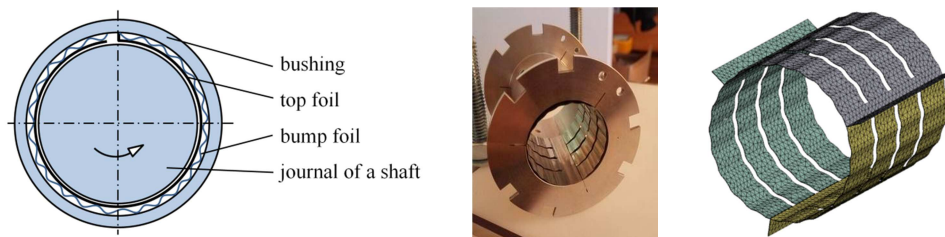
Fig. 1. Construction of a typical radial gas foil bearing (content from the applicants' reports): (a) example of its structure, (b) prototype - the bump foil is visible inside the bushing, (c) numerical model of a modular bump foil.
