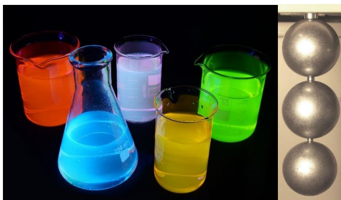
Figure 1. Fluorescence solutions under UV light illumination (left) and neodymium magnet that holds up to 1300 times its own weight (right).
