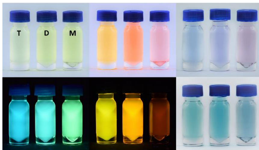
Figure 2. Our compounds change colors when dissolved in solvents of varying polarity: toluene (T), dichloromethane (D), and methanol (M).
