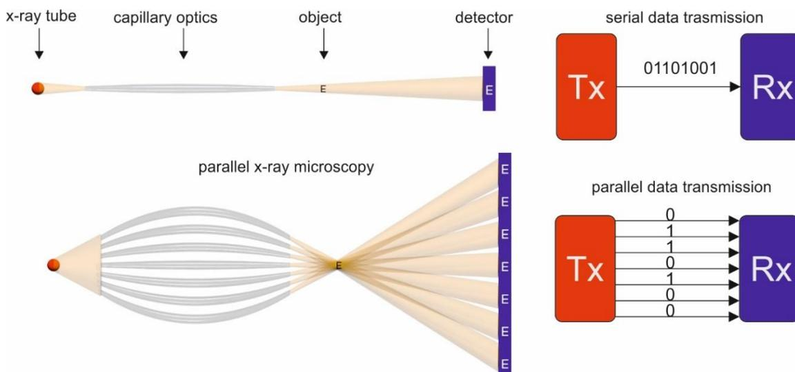
**Figure 2.** Analogy between parallel x-ray microscopy and parallel data transmission. In parallel x-ray microscopy the object is simultaneously imaged by multiple x-ray microbeams that are generated by tiny capillaries. Next, individual images are added numerically by means of computer software. Simultaneous detection of multiplexed x-ray images will result in much more efficient and faster x-ray laboratory based microscopy. In a similar way one increases speed of digital data transmission.
