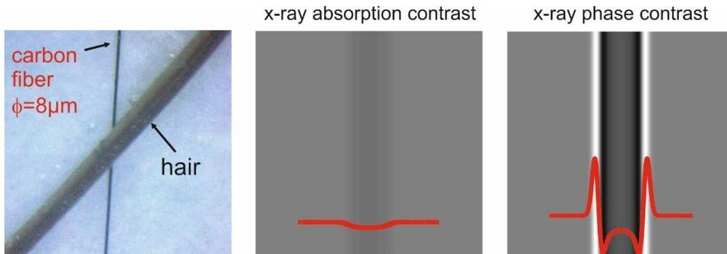
**Figure 1.** A carbon fiber (~8 times thinner than human hair) x-ray imaged with absorption and phase contrast (computer simulation). In the absorption image (contact geometry), the carbon fiber is hardly visible.
