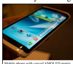
Mobile phone with curved AMOLED matrix
