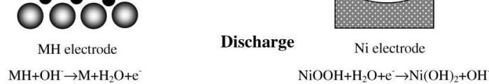
Fig. 2. Scheme of reactions occurring in a nickel-hydride battery during charging and discharging
