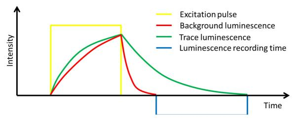
Fig. 1. Excitation, emission and delayed luminescence registration cycle.<sup>4</sup>
